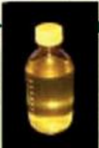
Corn syrup is a feedstock in the fermentation process, converted by microorganisms into Natural Plastics within the cell itself.
