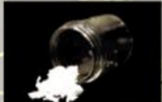
Dried polymer "crumb" is ready for pelletization.
